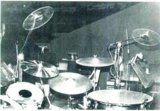
The microphone set-up, employing several PZM mics mounted on plexiglass disks, for the Ringling Bros. orchestra.
